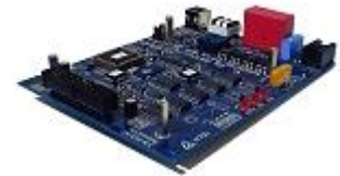
Above: The ThinkBoxx ST330 Telephone Module includes Programmable Dialer; Voice prompts with device readings and allows the user to switch devices on/off via the keypad of the mobile phone.
